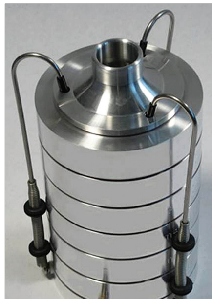
Widely used since the 1950s, the Andersen Cascade Impactor was, until recently, the gold standard for measuring particle size distribution from inhaled drugs or an air sample.
